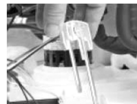
Electric conductivity-based water sensor
